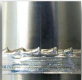
**Third Step**Entire application of a 0.2 mm thick protection and wear-resistant coating
